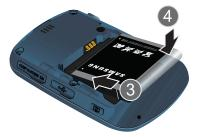
3. Insert the top end of the battery cover into the grooves of the phone. Snap the lid into place.
